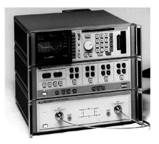
A photograph of the Hewlett-Packard HP8510B Network Analyzer. This test instrument is used to measure the scattering parameters (magnitude and phase) of a one ore two-port microwave network from 0.05 GHz to 26.5 GHz. Built-in microprocessors provide error correction, a high degree of accuracy, and a wide choice of display formats. This analyzer can also perform a fast Fourier transform of the frequency domain data to provide a time domain response of the network under test.
